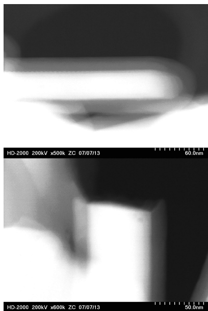
Figure 2. Z-contrast TEM images of Mo–V–Te–Nb–O M1 phase catalyst coated with alumina before crushing (top) and after crushing (bottom). The former image shows the complete coverage of the particle by alumina and the latter shows the exposure of ab plane at the top side of the particle after crushing.
